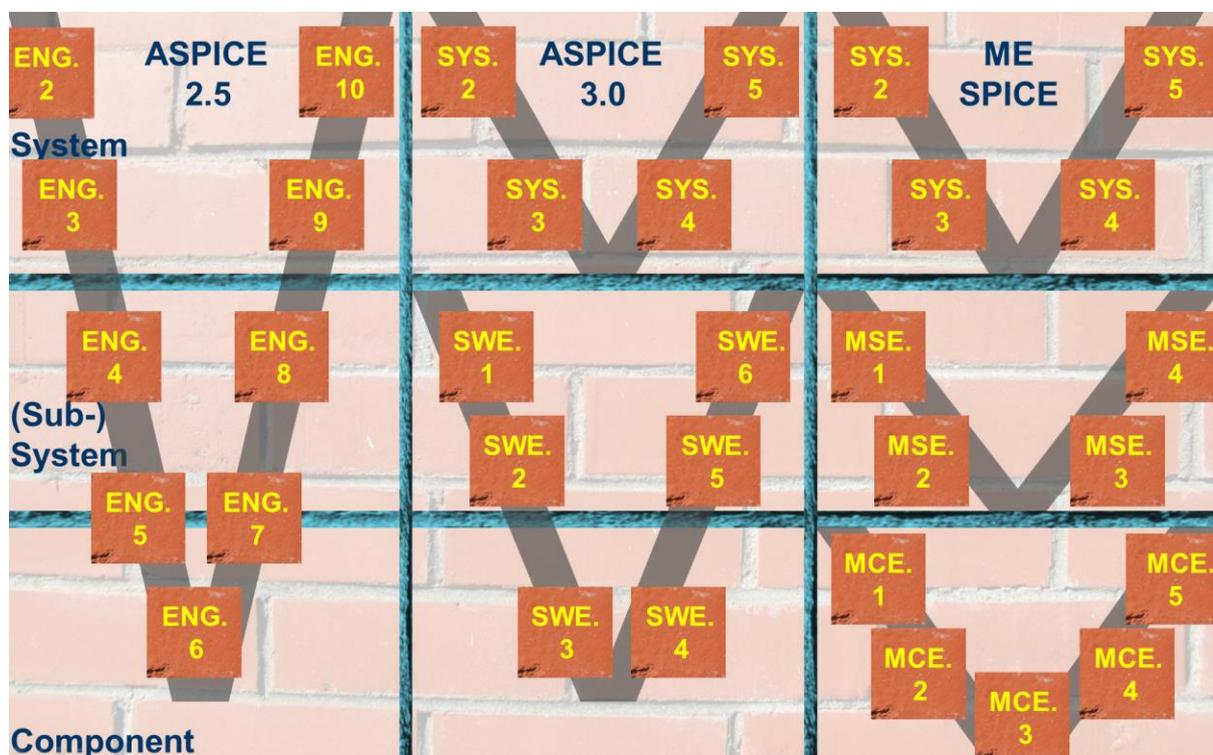
There is only an implementation process on the component level; the system is initially modelled on the subsystem level by use of further subsystems. In the mechanical area the "implementation" is the "creation of components". What a component actually is depends on several factors, like the production depth of the supplier, e.g. a component may be a gear wheel or an entire transmission.
